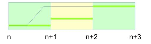
In the above graph, the thin line represents the input value and the green line the moving average. It can be seen that the moving average settles up to two periods after the input value has changed: any change occurred during the period starting at time 'n' is only completely accounted for at time 'n+2'.
